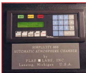
“PLC” Control Board
