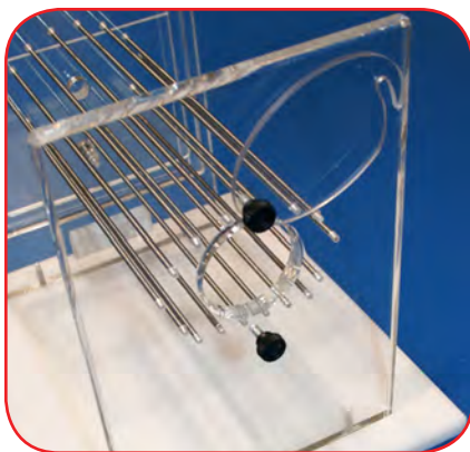
Close-up of rear locking door to prevent escape.
