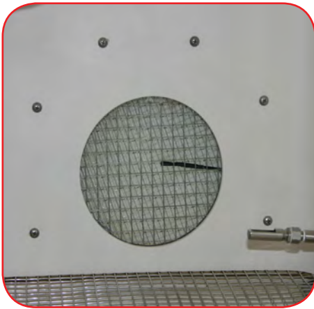
The thermocouple wire is inserted between the HEPA filter and inner cage wall.
