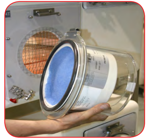
The blue "pre-filter" is placed in front of the exhaust HEPA filter. Place pre-filter on the outside of the air make up filter.
