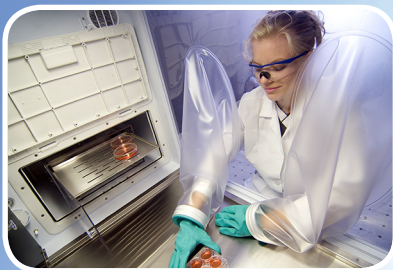
Soft, flexible glove fronts eliminate fatigue and discomfort caused by arms working in holes of hard fronts, without compromising visibility.
