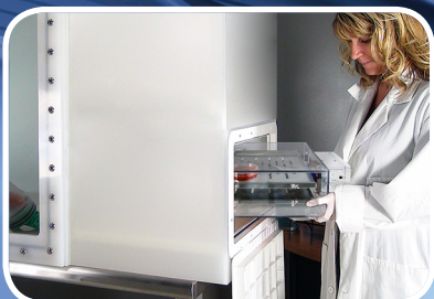
Buffer airlock also serves as docking chamber for transport chambers and remote subchambers allowing unlimited culture capacity.
