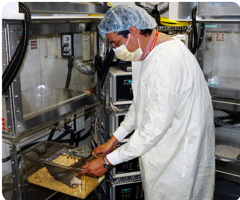
The A84XOV can be used in conjunction with other gas controllers to simulate the widest variety of conditions. Shown above, many chambers controlled by multiple BioSpherix controllers alongside an A84XOV.
