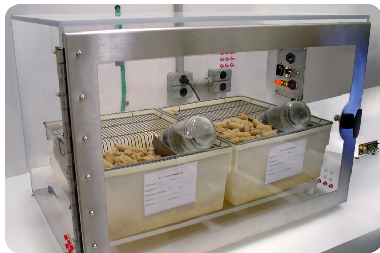
The ProCO 2 P120ppm works in semi-sealable chambers by forced displacement of gas via dilution with control gas. Pressure inside the chamber stays the same as pressure outside.
