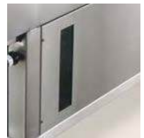
Waste tank viewing window
