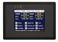
Microprocessor based I/O hardware with programmed logic running on Windows CE® platform. Control logic program is stored on a non-volatile, high capacity memory card EE-prom. All control parameter settings, alarms and setpoints are maintained during power failure, and restart is automatic upon power restoration.
