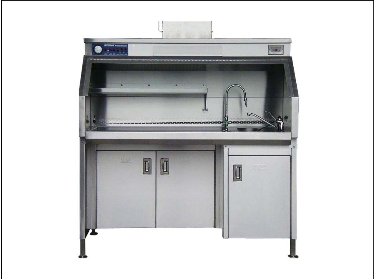
This 5 foot wide all stainless steel fume hood is specially designed for histology work from a sitting position. Adjustable legs allow it to be fixed at a wide range of heights. To positively control formaldehyde fumes this cabinet has a full wide front lip vent, two adjustable rear rents and a fully vented base cabinet.
